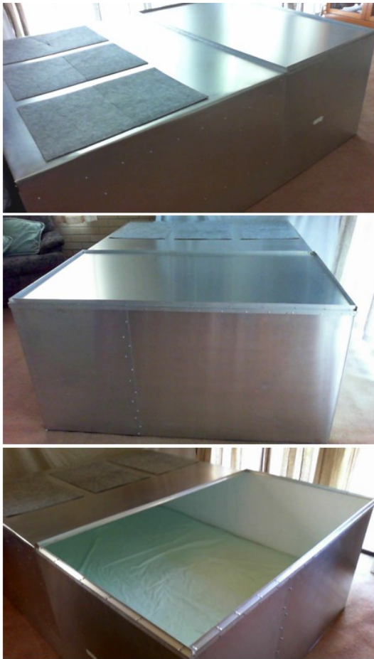
FIGURE 5. Various perspectives of a Faraday-type shielding cage housing a double bed size mattress, with and without removable lid.
